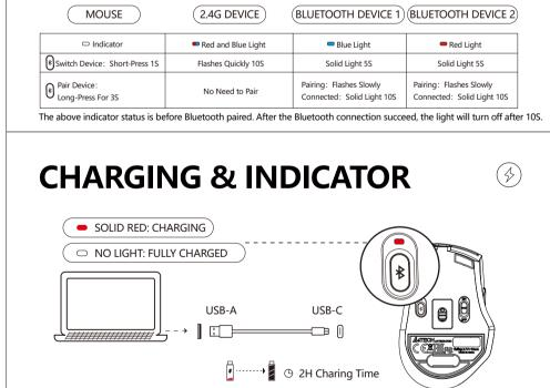
Flashing Red light indicates when the battery is below 25%.
